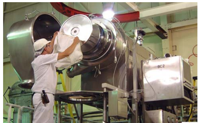
The Heinkel centrifuge in the flammable pilot plant is especially suited for nutraceutical extractions.
