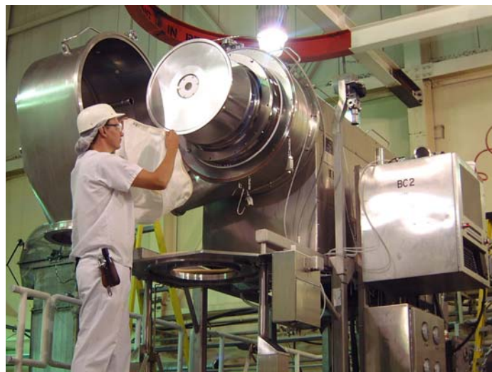
The Heinkel centrifuge in the flammable pilot plant is especially suited for nutraceutical extractions.
